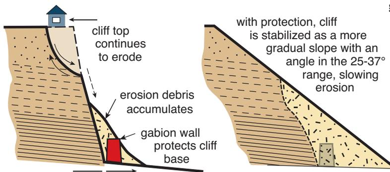
**Erosion can get you in two ways** on Calvert Cliffs, scientists have shown. Naturally eroding cliffs maintain a steep slope as they recede. Cliffs protected by erosion-stabilization efforts — like gabions — ideally, recede more slowly, becoming gentle slopes. Either way, houses that are too close to the edge may come tumbling down. ILLUSTRATIONS, ADAPTED BY SANDY RODGERS FROM FIGURES IN CLARK ET AL. 2004
