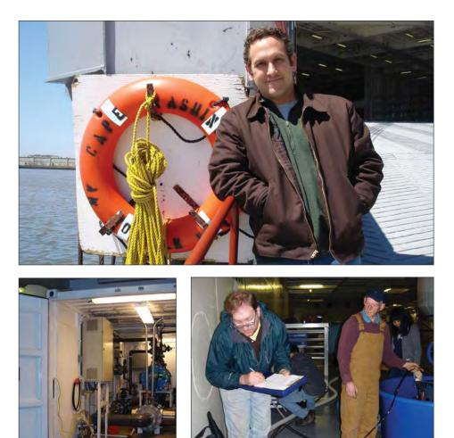
**Maritime Environmental Resource Center** director Mario Tamburri (top) oversees testing of ballast water treatment systems. New technologies come in large containers like the one housing the filter-UV apparatus (bottom left). George Smith tests treated water with a probe, while Tim Mullady records the results. The two Smithsonian Environmental Research Center biologists form part of a multi-institutional team studying how treatment systems affect ballast water. PHOTOS BY JESSICA SMITS.
