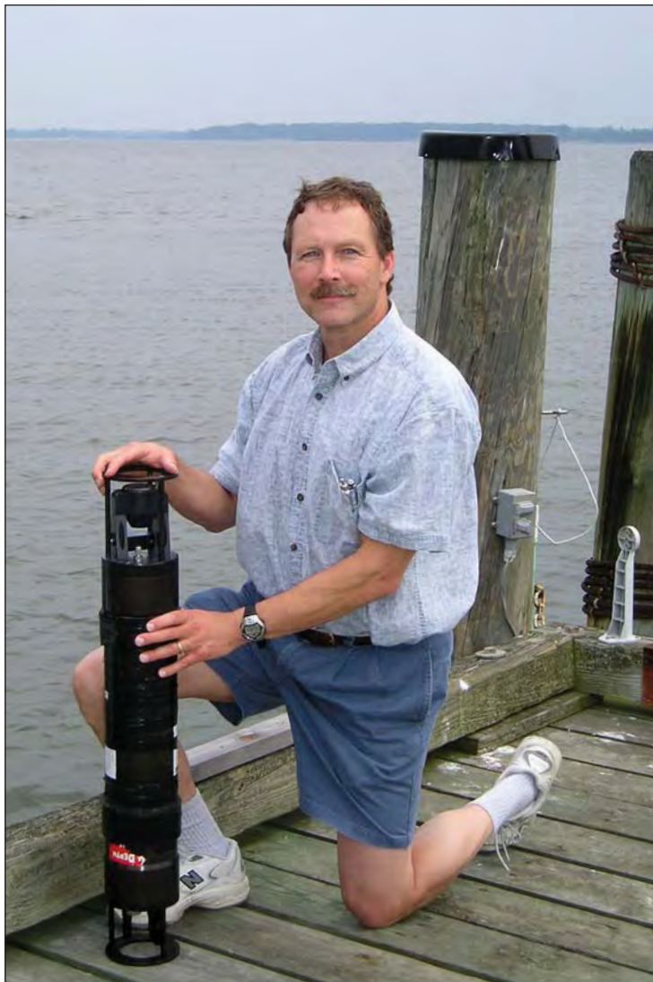
On the trail of sediment , researcher Larry Sanford holds a laser-shooting LISST, an instrument he uses to measure fine particles in the Bay. Looking like a cross between a robotic fish and a torpedo rack, the array he calls a DIPSTIC (above, right) carries a LISST on the back, as well as torpedo-like tubes and other instruments that capture snapshots of sediment all around the Chesapeake.
