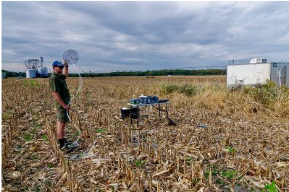
Jake Hagedorn, a doctoral student at the University of Maryland Center for Environmental Science's Appalachian Laboratory, employs a system to measure nitrogen gases that may be released as an unintended consequence of denitrifying practices. Photo, Brennen Jensen
