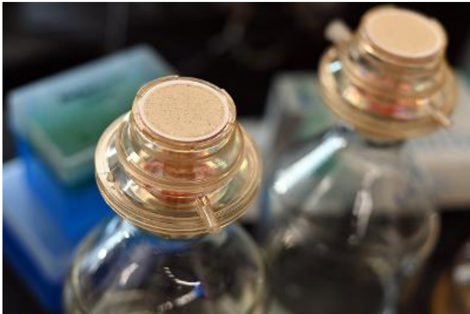
Water samples are pulled through filters, providing dissolved organic material to analyze.
