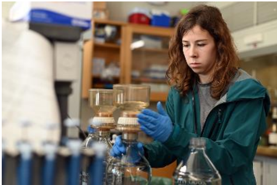
Graduate student Katie Martin filters creek water samples to extract and concentrate the dissolved organic components from them at University of Maryland Center for Environmental Science's Chesapeake Biological Laboratory.
