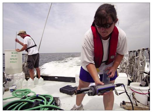
**Balancing on the deck** of the R/V Kerhin, Kristen Heyer shows off a probe used to monitor water quality in the Chesapeake Bay. The Maryland Department of Natural Resources crewmembers lower this probe via a metal cable down into the choppy Bay, taking detailed readings of temperature, saltiness, and dissolved oxygen levels up and down the water column. Those data points are later fed into a computer model of the Bay. PHOTOGRAPH BY DANIEL STRAIN.
